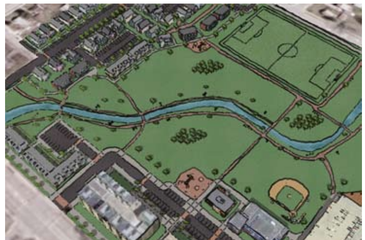
Using the most flood-prone areas as a park will create a strong attractor for the entire development.
